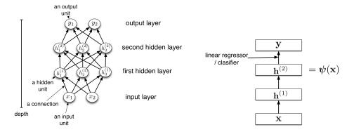
Figure 1: A multilayer perceptron with two hidden layers. **Left:** with the units written out explicitly. **Right:** representing layers as boxes.
