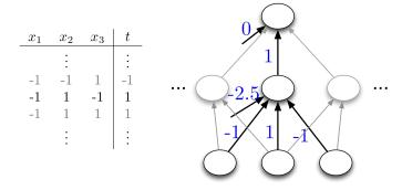
Figure 4: Designing a binary threshold network to compute a particular function.
